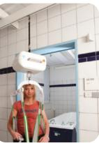
The lifting module has to be positioned close to the door header...
