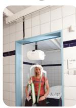
...Finally the other, inactive, strap needs to be detached and the lifting module can be moved on the next railing.
